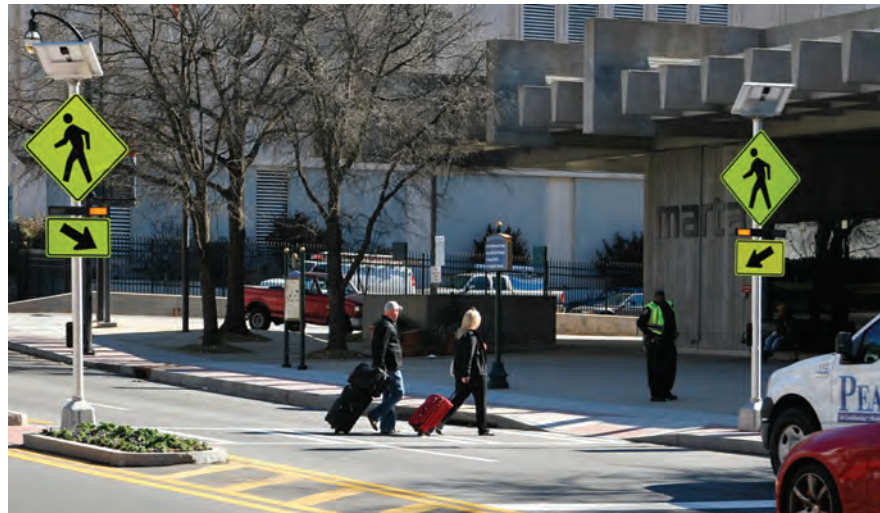
Rectangular Rapid Flash Beacons prompt more drivers to stop at crosswalks than other active treatments.
