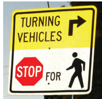
The R10-15 signs reminds drivers to stop to stop for pedestrians before turning.
