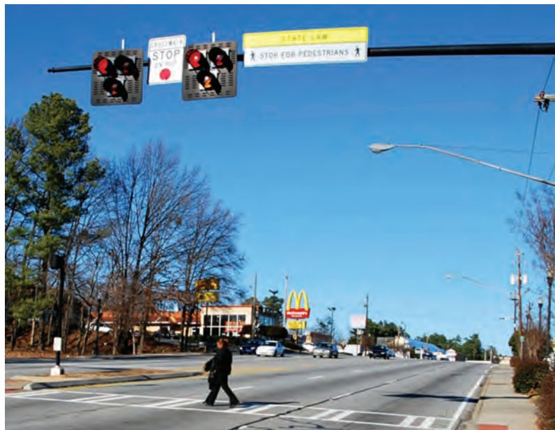
HAWK beacons are well-suited for mid-block crossings on high-speed, multi-lane roads.
