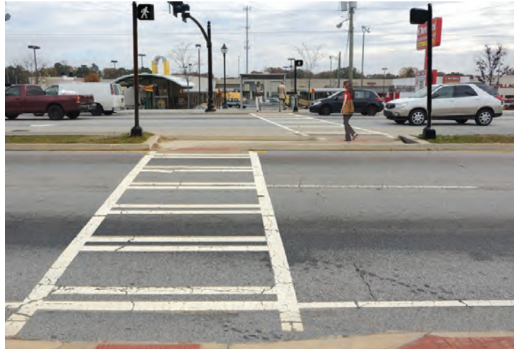
When used at locations with crosswalks, median refuge islands cut pedestrian crashes by 46 percent.
