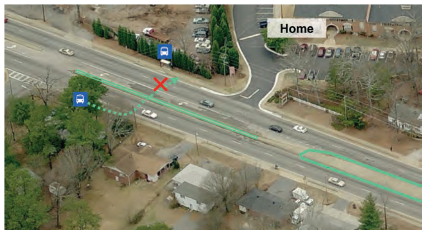
Relocating bus stops to places with medians is a low-cost way to increase safety.
